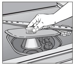
■ Lift the combination filter out of the machine. Remove any coarse particles and rinse it under running water. A nylon brush can be used, if necessary.
